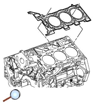
2. Install a NEW cylinder head gasket.
