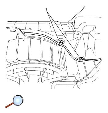
**Important:** Use a pair of long nose pliers to close the wiring harness retaining clip (1) ends to remove the wiring harness retaining clips (1) from the HVAC module assembly (2)
