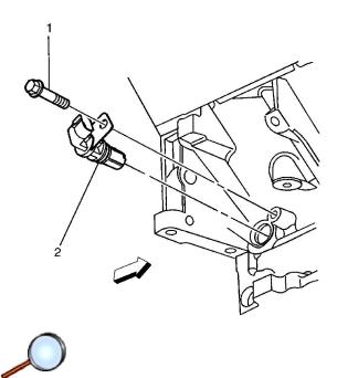
1. Install the CKP sensor (2) to the engine block.
