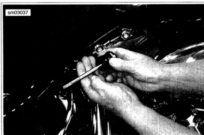
Figure 1-1. Checking Oil Tank Level
