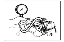
(c) Mount the joint and pressure gauge into the preheating plug hole of the first cylinder.
