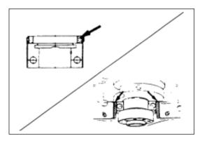
(i) Cover the fitting surfaces of fifth bearing cap and housing with recommended fluid sealant or its equivalent, shown in figure
