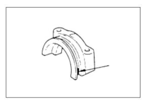
(h) Cover the fifth bearing cap of the crankshaft with recommended fluid sealant or its equivalent, shown in figure
