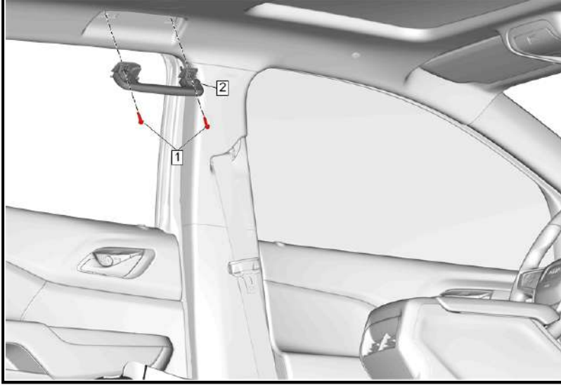
Roof Rail Rear Assist Handle (2) - Remove (Qty: 2) - Roof Rail Rear Assist Handle Replacement
