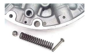
**Step 17:** Gently flat sand the passage walls of the pump, as well as the stator support passages if equipped, only enough to get rid of high spots around bolt holes and edges. Inspect all pump parts for wear or damage, replacing any bad parts you may find. Thoroughly clean all pump parts.
