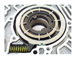
**Step 32:** Check the front stator bushing clearance between the bushing and the turbine shaft center journal. If it's not over 0.002", it can be re-used as long as the journal is in good shape.
