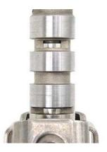
**Step 22:** Tap a new governor gear all the way into the shaft, making sure not to crack the new gear. Do not place the weight end of the governor against the bench while hammering on the gear. One suggestion is to hold the governor against your belt while tapping on the gear to absorb the shock.
