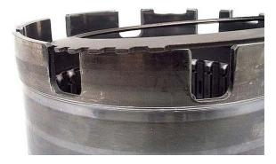
**Step 10:** Load the clutch plates into the drum, starting with a steel plate, ending with a friction plate.
