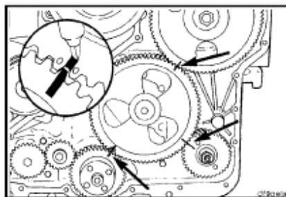
Use a felt marker to black the timing marks on the gear train. Use the marker to make alignment mark on the accessory drive gear and shaft.
