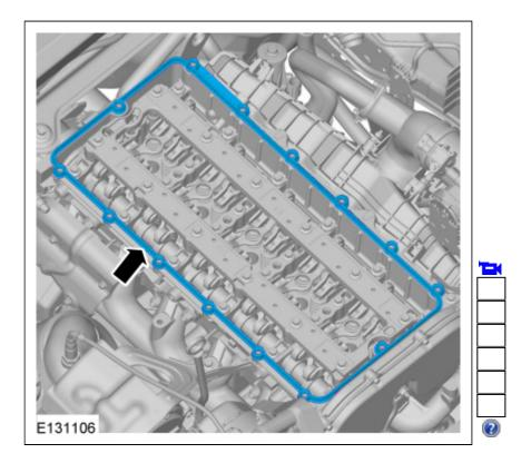
68. *Torque*: stage 1: 4 Nm stage 2: 10 Nm
