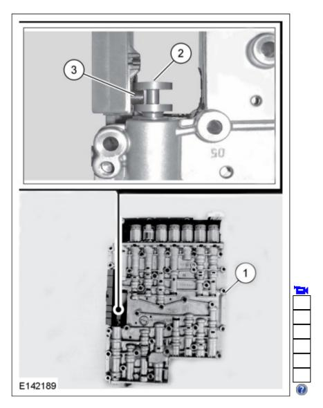
10. Install the 6 long molded leadframe-to-valve body bolts hand-tight.
