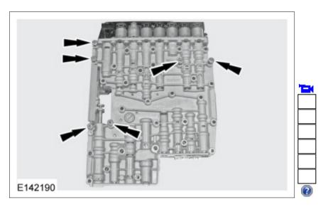
11. Install the 19 short main control assembly lower-to-upper valve body bolts. Tighten the bolts in the sequence shown.
