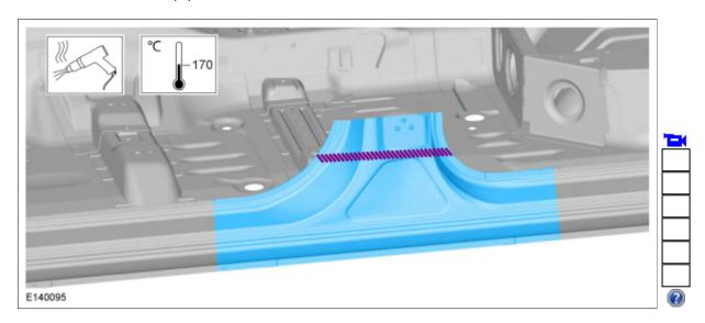
• Use the General Equipment: Spot Weld Drill Bit
