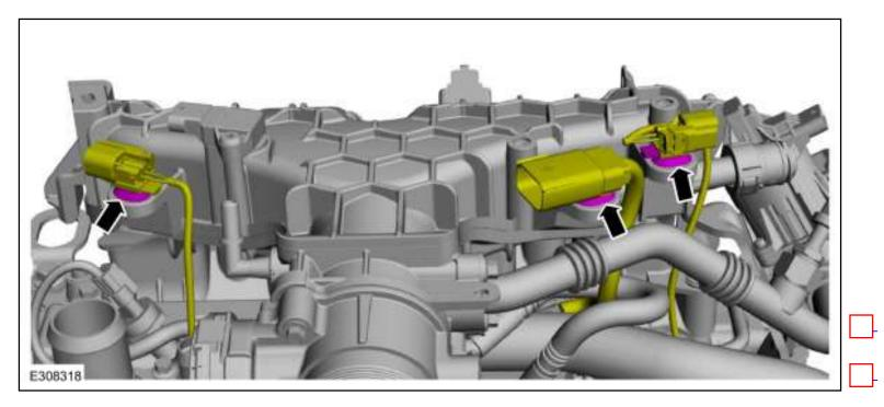
169. Install the ground cable and the bolt. *Torque* : 133 lb.in (15 Nm)
