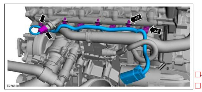
168. Attach the wiring connector retainers to the intake manifold.
