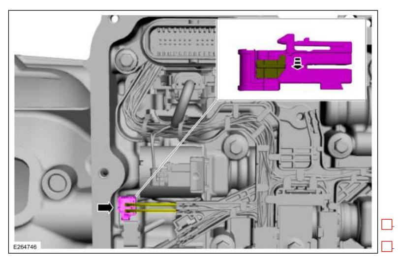
26. Unlock and disconnect the TR sensor electrical connector.
