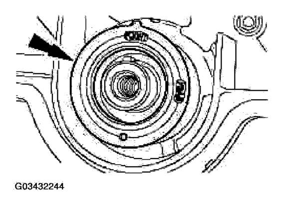
Fig. 196: Installing Crankshaft Timing Belt Pulley Courtesy of FORD MOTOR CO.
