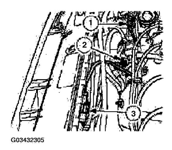
Fig. 257: Disconnecting Electrical Connectors Courtesy of FORD MOTOR CO.
