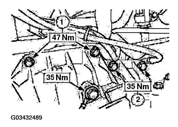
Fig. 441: Installing Transaxle Upper Flange Bolts And Starter Motor Bolts Courtesy of FORD MOTOR CO.
