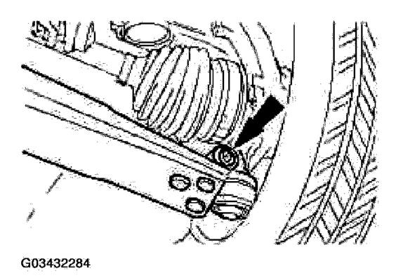
Fig. 236: Removing Suspension Arms Courtesy of FORD MOTOR CO.
