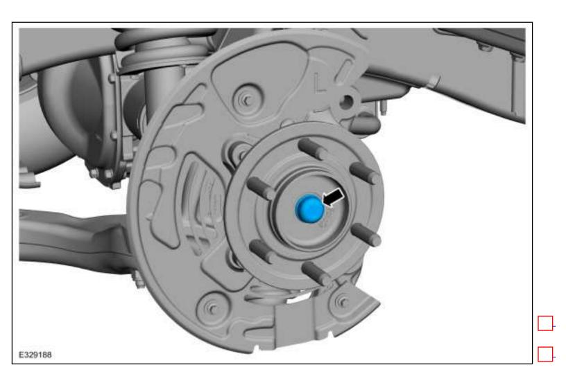
6. NOTICE: When installing the halfshafts measure the depth of the CV shaft threaded end to the inner bearing race. The minimum depth is 15.5 mm (0.61 in). If the depth is less than 15.5 mm (0.61 in) rotate the CV shaft to clear a binding condition between the IWE and CV splines. Installing the axle nut and tightening without the proper depth of protrusion will result in damage to the IWE.
