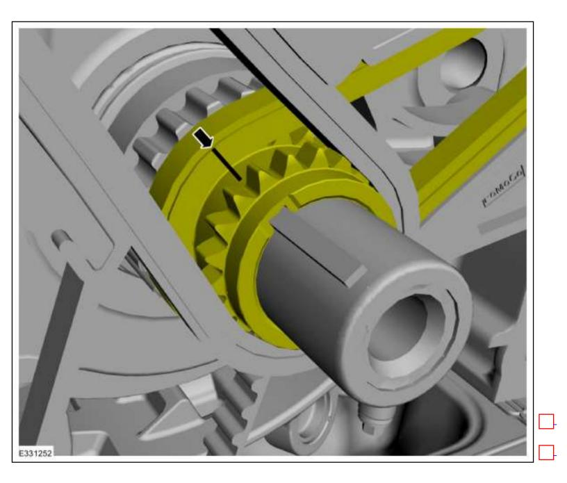
3. NOTICE: The timing chain must remain in its original position on the VCT unit using the scribed marks, or damage to valves and pistons will result.
