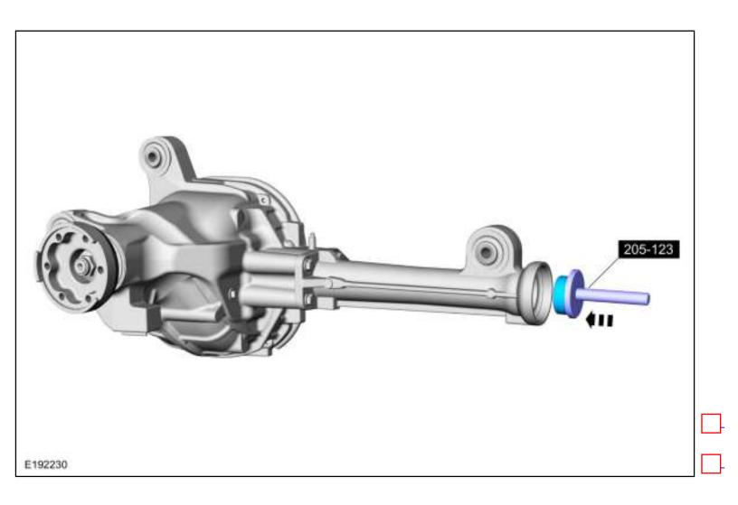
2. Install the axle shaft seal.
