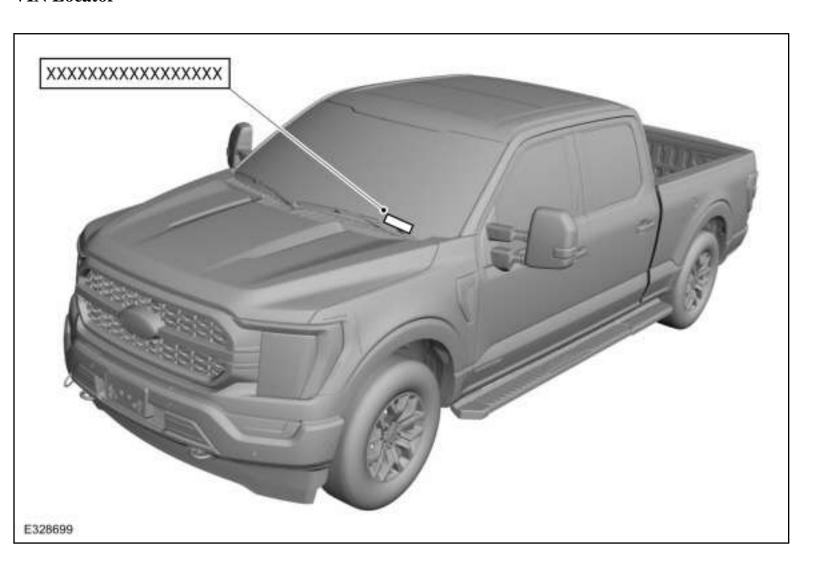
The VIN is a 17-digit combination of letters and numbers. The VIN is stamped on a metal tab riveted to the instrument panel, top upper left of the dash. The VIN is also found on the VC label. If the VIN plate requires replacement, authorized dealers must contact their respective regional office.
