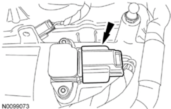
Fig. 96: Locating Manifold Absolute Pressure (MAP)/Intake Air Temperature 2 (IAT2) Sensor Electrical Connector Courtesy of FORD MOTOR CO.
