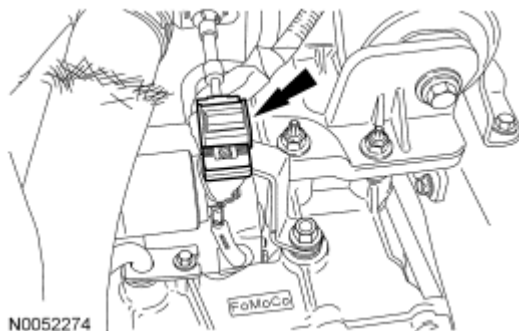
Fig. 434: Locating Selector Lever Cable End From Manual Lever Courtesy of FORD MOTOR CO.
