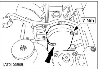
**5. NOTE:** Fit the bracket for the cable tie for the starter motor wiring.
