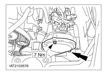
13. Fit the injection pump timing belt cover.
