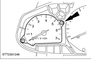
3. Remove the tachometer.
