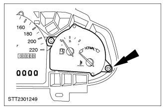
4. Remove the fuel / temperature gauge.
