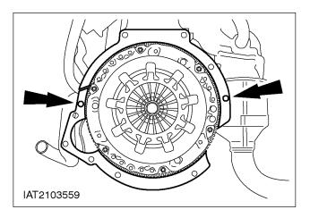
**2. NOTE:** Make sure the guide sleeves are correctly seated.
