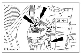
17. CAUTION: Position the generator and screw in the bolts finger tight. First tighten the bolt on the pulley side, then the rear upper long bolt and finally the rear lower short bolt.
