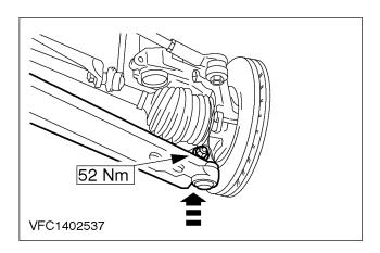
5. Attach the lower suspension arms to the spindle carriers.
