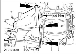
**3. NOTE:** The transmission is centered with two guide sleeves on the engine.
