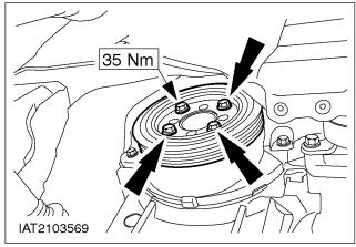
16. Fit the crankshaft pulley/vibration damper.
