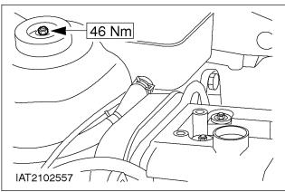
**8. NOTE:** Use an Allen key to stop the piston rod from turning.
