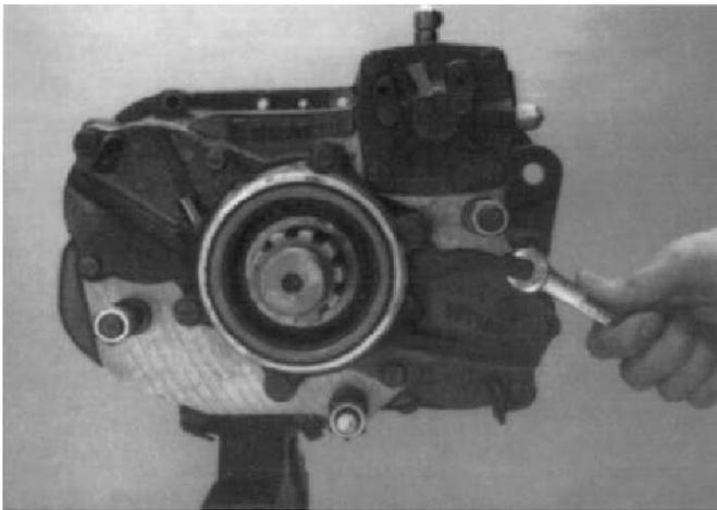
2. If necessary, remove the oil seal from the rear bearing cover.
