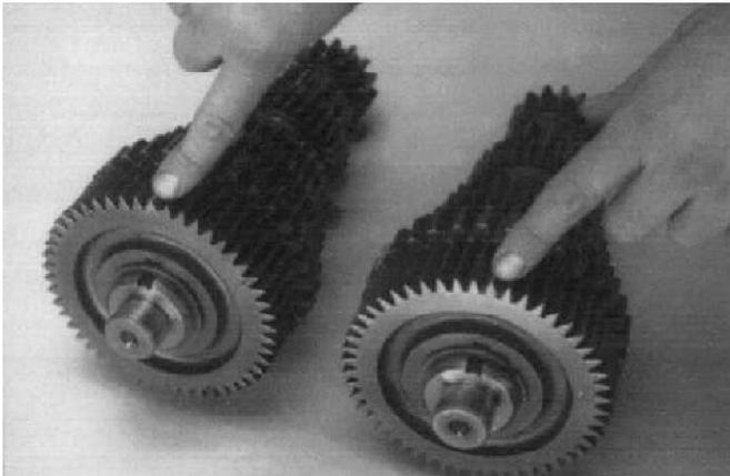
5. Install the snap ring in each countershaft front groove.
