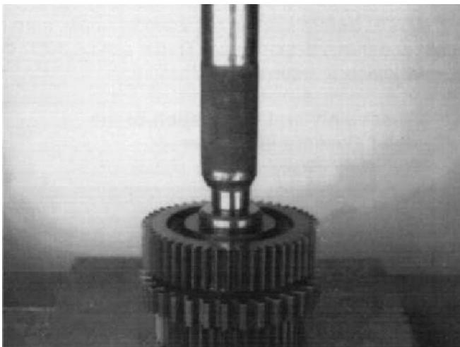
4. If necessary, remove the countershaft key.
