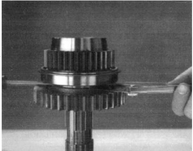
8. After proper reverse gear clearance has been set, remove the snap ring from the mainshaft rear, remove the auxiliary drive gear and the reverse gear from the mainshaft. The tolerance washer and key remain on the mainshaft. Reposition the mainshaft with the reverse gear minus its snap ring in the vise as shown, pilot end up, with the keyway accessible.
