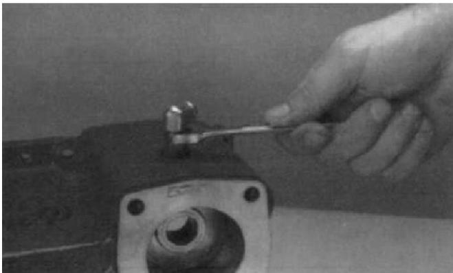
10. Remove the cylinder housing.
