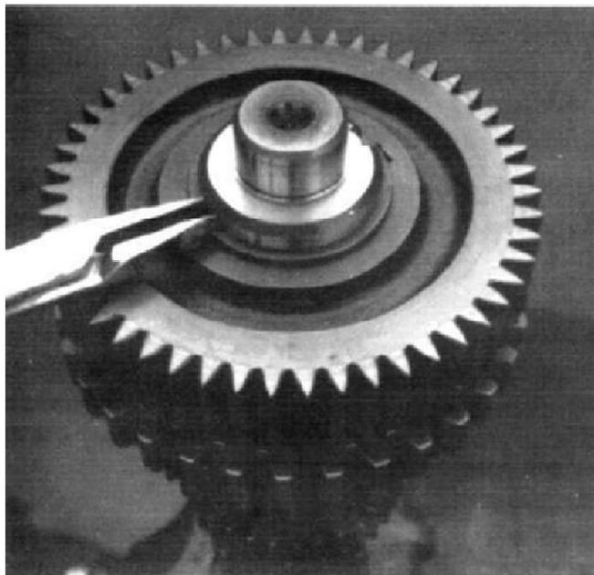
3. Remove countershaft drive gear, countershaft PTO gear, and countershaft 3rd speed gear together by pressing on the countershaft 3rd speed gear bottom face.
