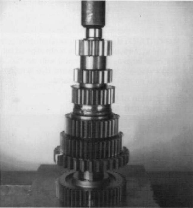
4. Align the countershaft drive gear keyway with countershaft key, press the countershaft drive gear onto the countershaft with gear long hub to the rear, (marked timing tooth to the front.)
