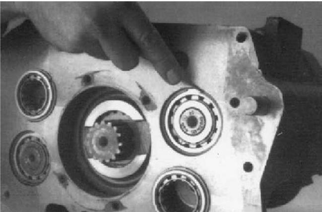
1. Remove the upper countershaft snap ring from the case rear bearing bore.
