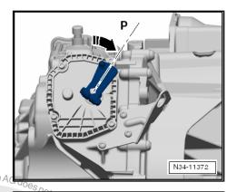
Install Bowden cable with loosened adjusting screw -arrow-and new securing clip and new securing clip.
