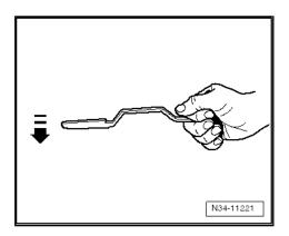
Remove securing clip in -direction of arrow-.
