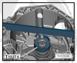
Place digital depth gauge "at top" onto outer input shaft. oo to open in in it is in it i
