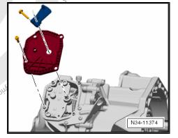
Working through opening, push selector fork to side -direction of arrow-.
