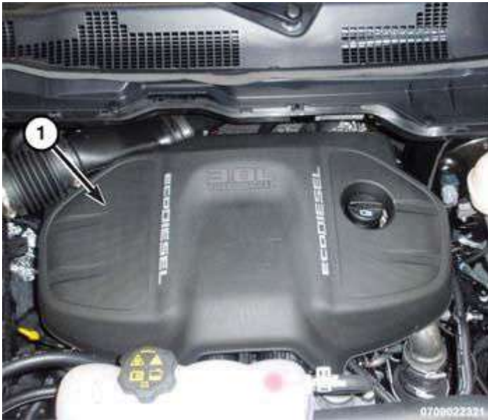
Fig. 465: Removing/Installing Engine Cover Courtesy of CHRYSLER GROUP, LLC
