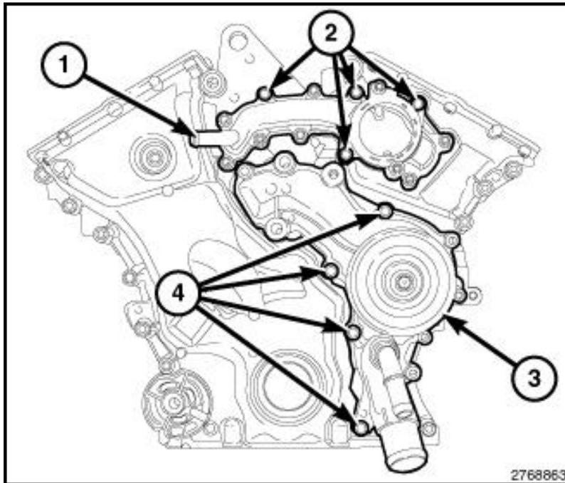
2. Remove the heater supply hose from the coolant crossover (1).
