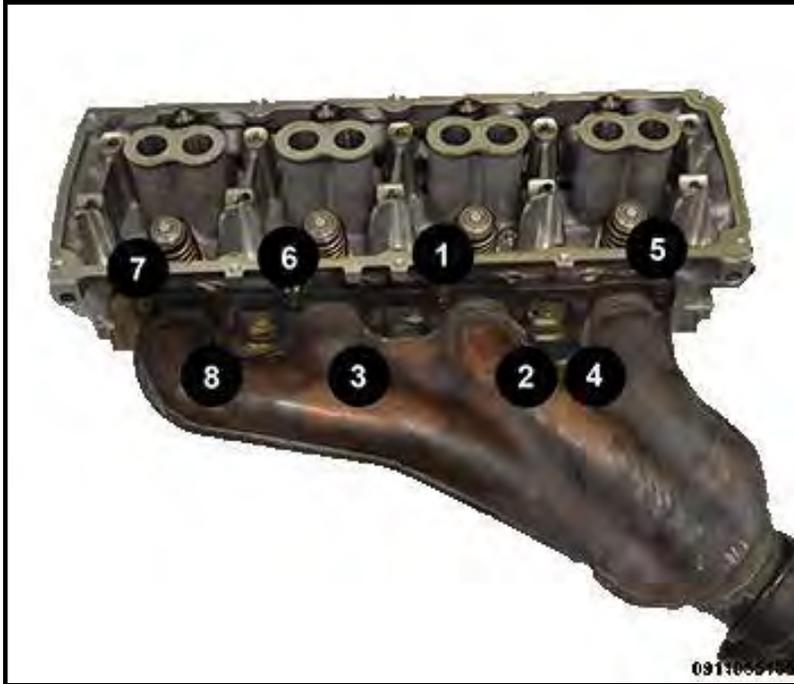
3. Remove the exhaust manifold bolts using the sequence shown in illustration, starting at eight and going backwards.
