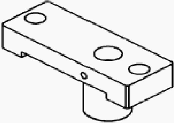
A perspective view of a rectangular gage plate. It has three circular holes on its top surface and a cylindrical base protruding from the bottom center.                                                                                           | <p>9681-2 - Plate, Gage (Originally Shipped In Kit Number(s) 9674.)</p>          |
