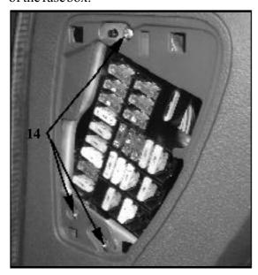
Remove the access cover to the fuse box. Swingover the littlecaps from the dashboard lowerpart and dismount the attachments crews (15) on the driving post cross member.
