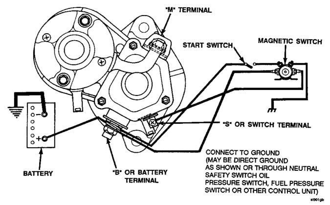
Basic Wiring Circuit (with auxillary magnetic switch)
