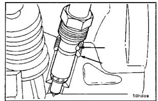
Assemble the fuel drain manifold and high pressure lines. Leave the high pressure fittings loose at the injectors.
