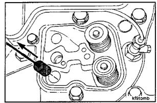
Install a wooden dowel into the top of the tappet. Wrap rubber bands around the wooden dowels to secure the tappets.
