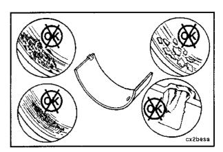
Visually inspect the bearing shell seating surface for nicks or burrs.
