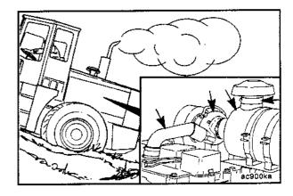
Check the intake air system for leaks. Make sure a sealant is used on the through-hole capscrews which secure the manifold cover to the head.
