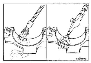
Visually inspect the connecting rod caps, connecting rod bearing saddles, and capscrews for nicks, cracks, burrs, scratches, or fretting.
