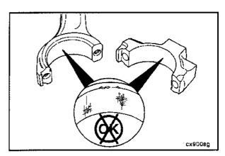
Visually inspect the bearings for damage.
