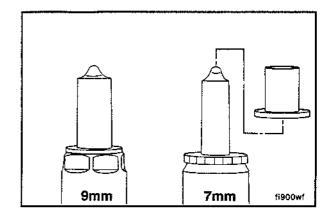
Apply a coat of anti-seize compound to the threads of the injector hold down nut and between the top of the nut and injector body.
