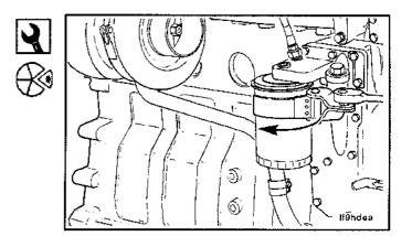
Clean around the lubricating oil cooler cover.
