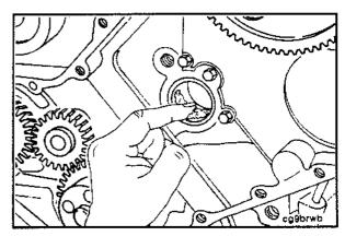
Lubricate the camshaft lobes, journals and thrust washer with Lubriplate™ 105.
