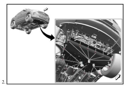
Front Compartment Insulator - Remove - <u>Front Compartment Insulator Replacement (Base)</u>, or <u>Front Compartment Insulator Replacement (Service Cover for Engine Oil Filter)</u>, or <u>Front</u> <u>Compartment Insulator Replacement (Service Cover for Engine Oil Drain)</u>
