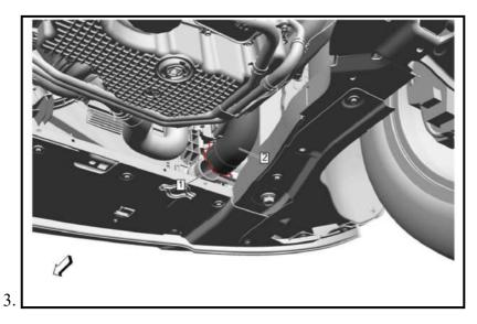
Charge Air Cooler Outlet Air Hose Retainer Spring (1) - Remove
