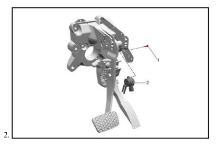
Brake Pedal Position Sensor Bolt (1) - Remove
