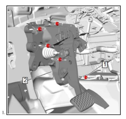
Brake and Accelerator Pedal Assembly (2) - Remove - <u>Brake and Accelerator Pedal Assembly</u> <u>Replacement</u>
