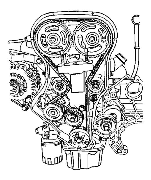
Fig. 18: View Of Timing Belt And Components Courtesy of GENERAL MOTORS CORP.
