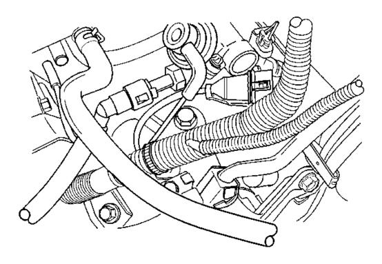
Fig. 5: View Of Surge Tank Coolant Hose Courtesy of GENERAL MOTORS CORP.
