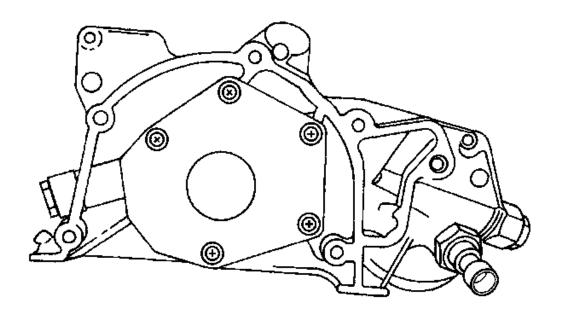
Fig. 103: Rear View Of Oil Pump Courtesy of GENERAL MOTORS CORP.
