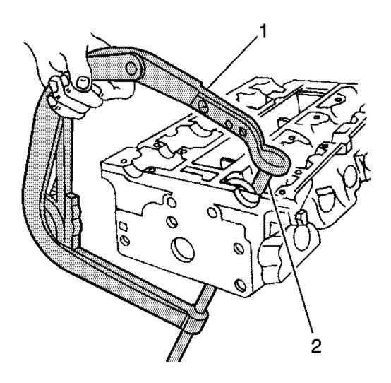
Fig. 194: Compressing Valve Springs Courtesy of GENERAL MOTORS CORP.
