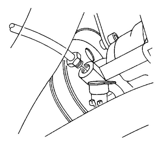
Fig. 118: View Of Power Steering Pressure Hose Courtesy of GENERAL MOTORS CORP.
