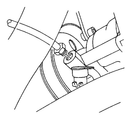
Fig. 134: View Of Power Steering Pressure Hose Courtesy of GENERAL MOTORS CORP.
