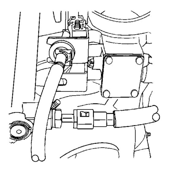
Fig. 67: View Of Fuel Return Line And Fuel Feed Line Courtesy of GENERAL MOTORS CORP.
