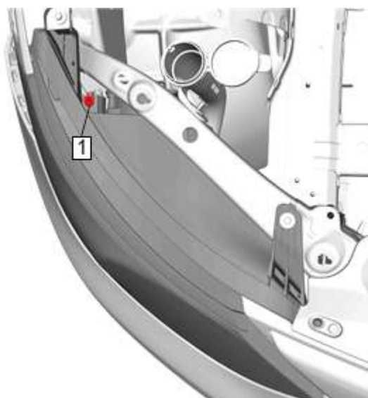
Fig. 32: Vertical Aim Screw Courtesy of GENERAL MOTORS COMPANY
