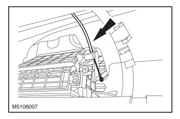
3 Disconnect the A/C mode vent control cable (1) and A/C temperature vent control cable (2).
