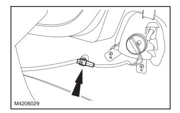
**4.** Remove 3 retaining screws from the rear fog lamp, and remove the rear fog lamp.
