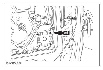
**5.** Disconnect the speaker wiring harness connector, and remove the speaker.
