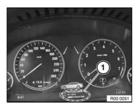
The status of the reset is indicated in the display by a progress bar and in text as "Reset running" (1).
