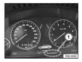
Confirm text message "Execute reset?" (1) by pressing the button for 3 seconds again.
