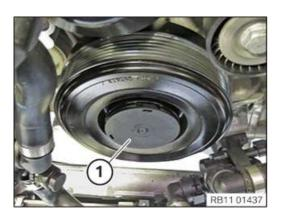
Release cover (1) from the vibration damper with a screwdriver.
