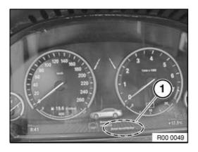
If a reset is possible, this is displayed in the instrument panel as "Reset executable" (1).
