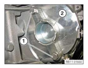
Release screws (1) from the transportation retainer (2).
