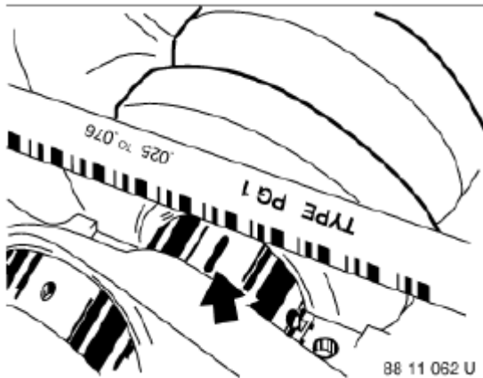
Fig. 156: Checking Main Bearing Play Courtesy of BMW OF NORTH AMERICA, INC.
