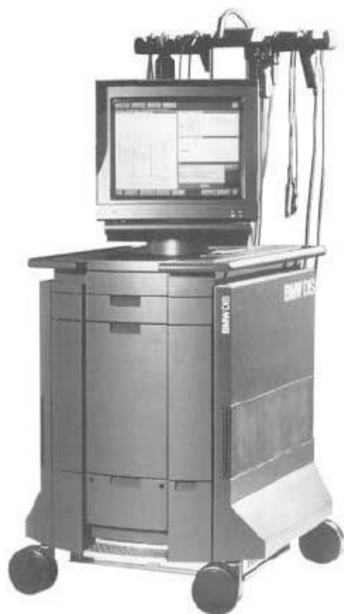
Fig. 9: Identifying BMW Diagnosis Information System (DIS)
