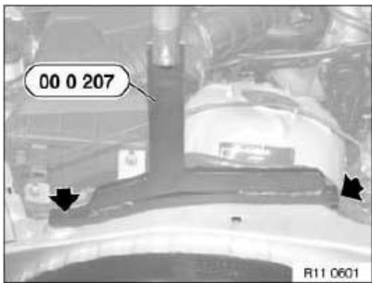
Fig. 88: Identifying Special Tool (00 0 207)
