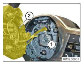
• Connect and lock the connector (1) of the airbag unit (2).
