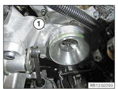
Check the sealing ring (1) on the exhaust turbocharger for damage and renew if necessary.
