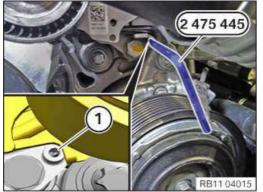
Guide in the special tool <u>2 475 445</u> and install it in the bore hole (1).
