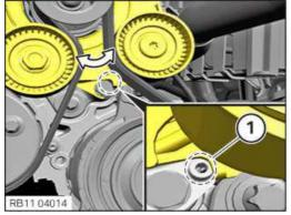
• Position the belt tensioner so that the bore hole is visible in the area (1).
