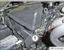
• Feed in and install clean air pipe with resonator (1) in the direction of the arrow.
