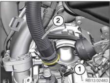
Check the sealing ring (1) for the engine ventilation line (2) for damage and renew where required.
