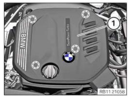
Unclip the acoustic cover (1) from the holders in the indicated area towards the top.
