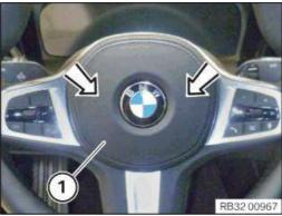
Press the airbag unit further (1) with even pressure in the direction of the arrow into the steering wheel.
