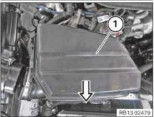
• Press and hold clean air pipe with resonator (1) in the direction of the arrow.
