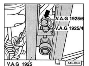
Insert VAG1925 spacer together with VAG1925/4 adapters and screw both threaded spindles out...
