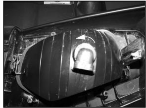
3. Insert new bulb. Reinstall the harness assembly into the headlight assembly.
