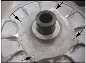
Place the clutch into the Clutch Compression Tool PN 8700220. Using Compression Extensions PN PS-45909, press down on top of the spider assembly, compressing the spider onto the shaft. Remove snap ring (A) and slowly release the assembly.
