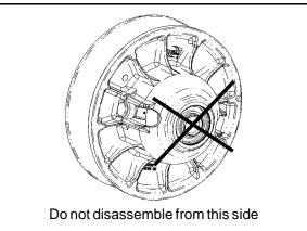
2. It is important to mark the position of the shaft, cam cover, and sheave before disassembly or use the X's on the components for reference. This will aid in reassembly and helps to maintain clutch balance after reassembly.
