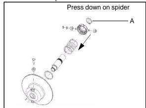
5. Remove the spider assembly, spring (B), and spacer washer (C).
