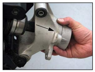
9. Rotate bearing by hand and check for smooth rotation. Visually inspect bearing for moisture, dirt, or corrosion.
