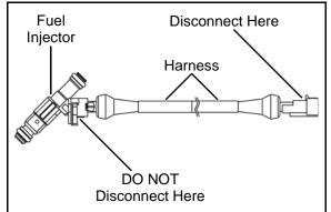
The fuel injectors are non-serviceable. If fault code diagnosis indicates a problem with either injector, test the resistance of the fuel injector(s) by measuring between the two harness pin terminals:
