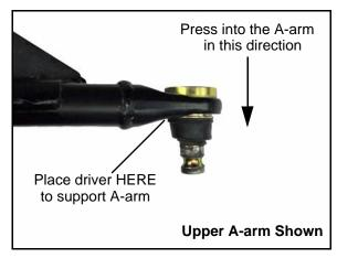
2. After the new ball joint is installed into the A-arm, install a NEW retaining ring.
