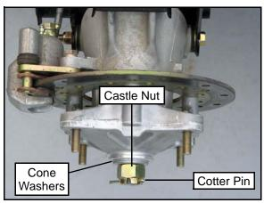
Remove the two brake caliper attaching bolts.
