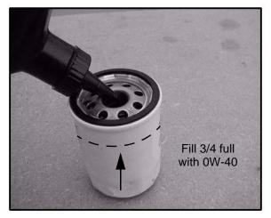
Remove primer plug from the engine. Install Oil System Priming Adapter (PU-45778) into the oil plug hole. Push 3-5 oz. (approx.) of Polaris 0W-40 into the adapter or until resistance is felt. Remove the adapter. Apply sealant to the plug threads. Install the plug and torque to specification.
