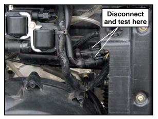
Fuel Injector Resistance Specification:  $13.8\Omega - 15.2\Omega$
