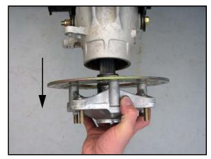
7. Remove the bolts that attach the rear bearing carrier to the upper and lower A-arms.
