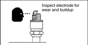
8. Clean with electrical contact cleaner or a glass bead spark plug cleaner only. **CAUTION:** A wire brush or coated abrasive should not be used.
