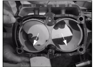
4. Inspect cylinder for taper and out of round with a telescoping gauge or a dial bore gauge. Measure in two different directions, front to back and side to side, on three different levels (1/2, down from top, in the middle, and 1/2, up from bottom). Record measurements. If cylinder is tapered or out of round beyond .002", the cylinder must be replaced.
