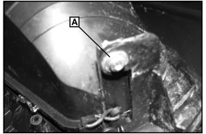
6. Adjust the beam to desired position. Repeat the procedure to adjust the other headlight.
