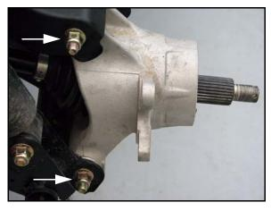
8. Remove the bearing carrier from the rear drive shaft.
