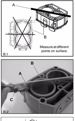
3. Inspect cylinder for wear, scratches, or damage.
