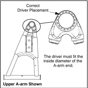
NOTE: The driver must fit the ball joint housing in the A-arm. This will allow the ball joint to be properly pressed out of the A-arm without damaging the Aarm.
