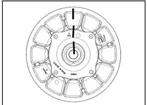
3. Remove the four torx screws that secure the cam (helix) assembly using a T25 torx driver.
