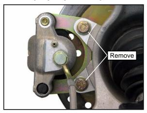
6. Remove the rear wheel hub assembly.
