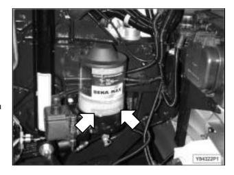
If the tank is empty, the driver's display also indicates the "central lubrication" symbol and the text "INFO ERROR GREASE CENT.LUBR.".
