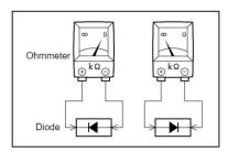
If the circuit has diodes, reverse the two leads and check
