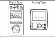
(c) Use a volt/ohmmeter with high impedance (10 k $\Omega/V$  minimum) for troubleshooting of the electrical circuit.
