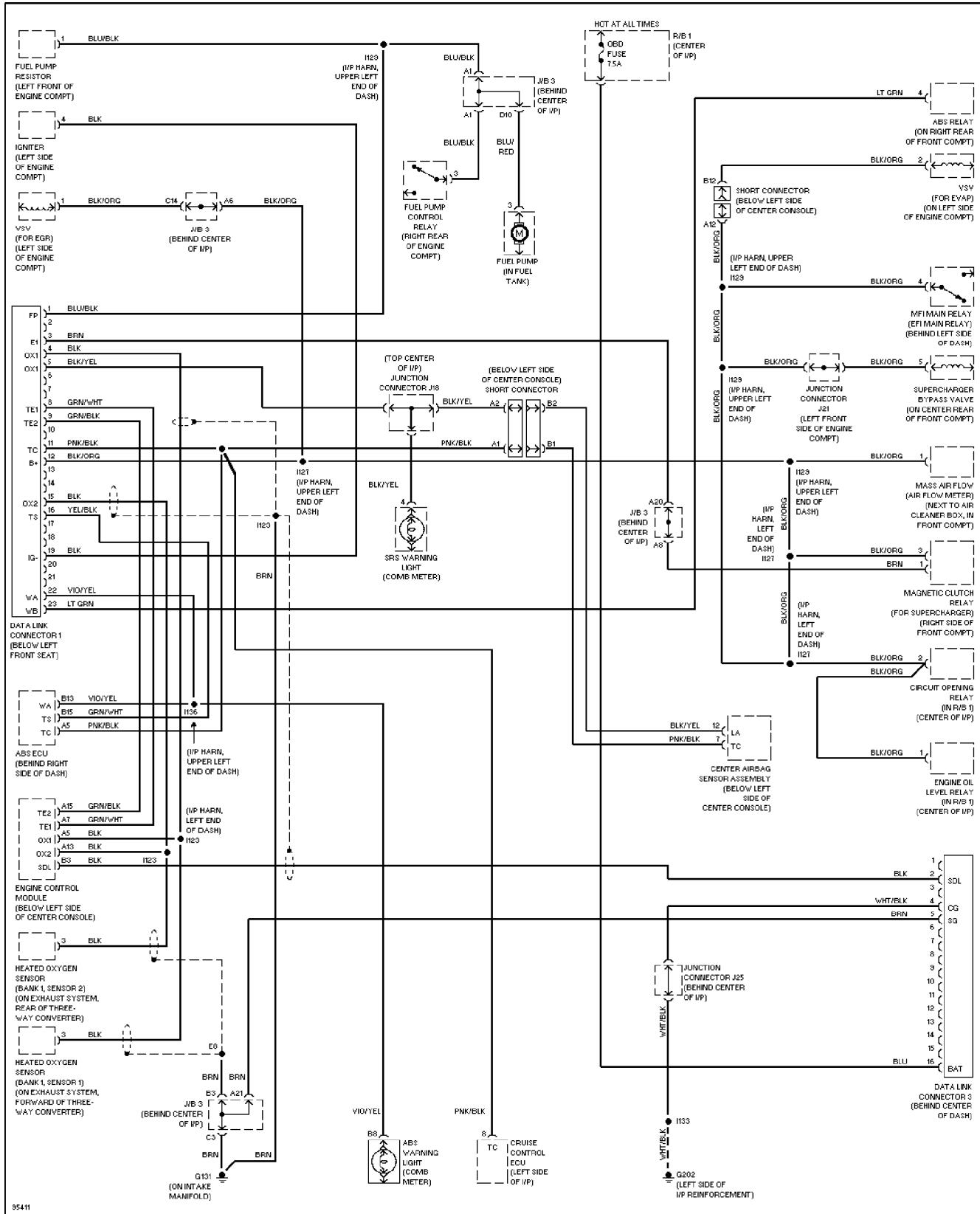
**SYSTEM WIRING DIAGRAMS**
