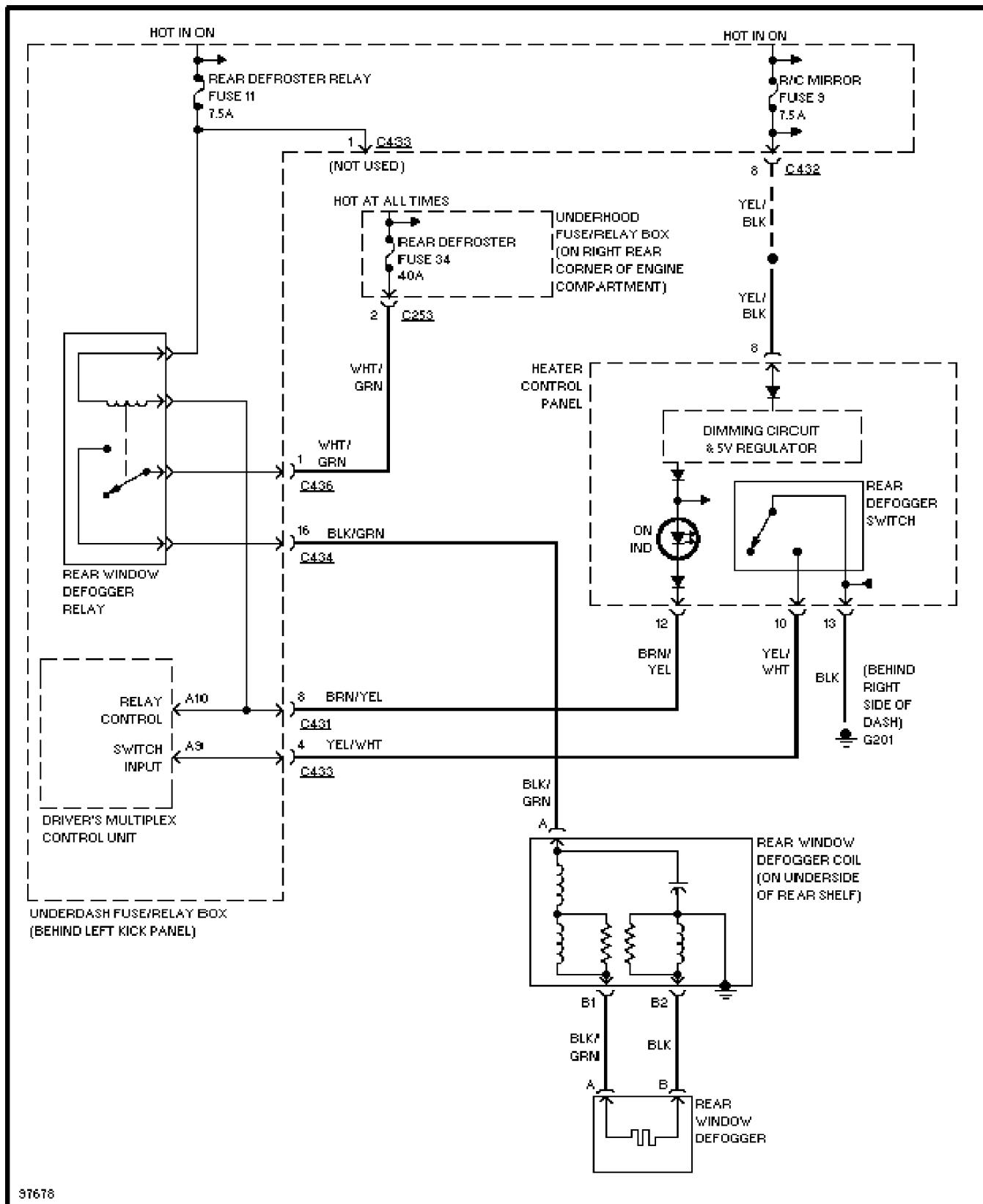
**SYSTEM WIRING DIAGRAMS**
