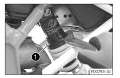
Adjust the spring preload by turning adjusting ring ①.
