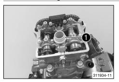
Grease the O-rings and mount spark plug shaft insert 1.
