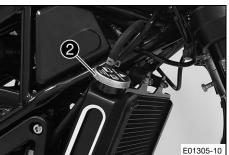
Remove radiator cap 2 and check the coolant level in the radiator.
