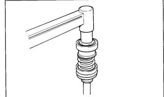
Coat the new O-rings and piston ring with clean shock oil or silicone grease.
