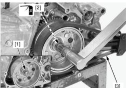
Apply engine oil to the starter reduction gear [1] journal and gear teeth.
