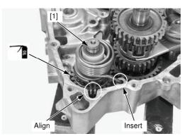
Set the retainer [1] to the kickstarter spindle.
