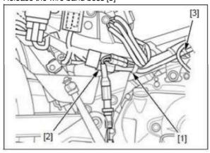
Disconnect the EOT sensor 2P (Black) connector [1] and release the EOT sensor wire [2] from the clamps [3].
