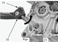
snap ring is firmly seated in the groove.
