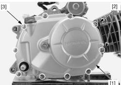
Install the kickstarter pedal [1] to its original position as marked during removal. Install and tighten the bolt [2].
