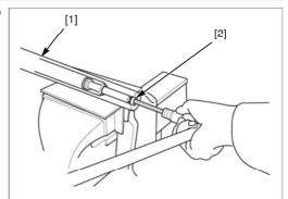
Remove the fork cap bolt [1], O-ring [2] and fork spring [3] from the fork pipe [4].
