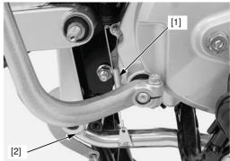
Remove the brake pedal return spring [1] from the brake rod and swingarm.
