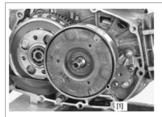
Remove the clutch lifter bearing [1].
