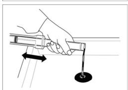
Remove the socket bolt [1] and sealing washer [2].
