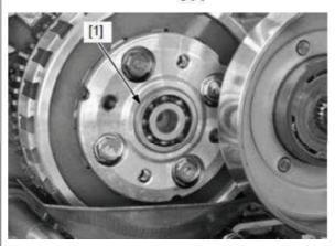
Hold the clutch lifter plate and remove the clutch center lock nut [1] using the special tools.
