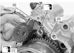
Apply engine oil to the starter reduction gear shaft [1]. Install the shaft into the reduction gear.
