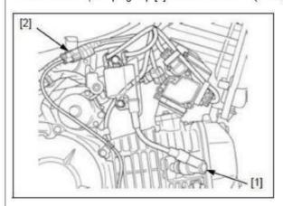
Remove the wire band [1] and disconnect the starter motor 2P connector [2].
