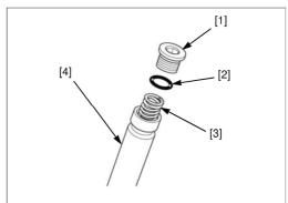
Pour out the fork fluid by pumping the fork pipe several times.
