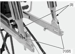
Remove the swingarm pivot bolt [1] and swingarm [2].
