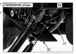
Disconnect the following from the EVAP canister [1]:
