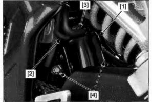
Remove the heat guard [1] by releasing the tabs [2] from the grooves of the rubber mount [3].
