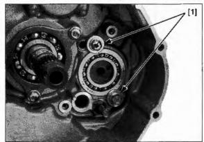
Remove the shift fork shaft [1] and shift forks [2].
