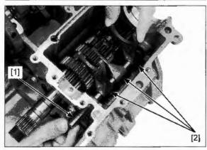
Remove the shift drum [1]/bearing [2] assembly. Remove the shift drum bearing from the shift drum.
