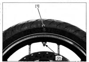
Note the rotating direction (arrow) marks [1] on the tire and wheel upon tire mounting. Always mount the tire onto the wheel with the marks facing in the same direction.
