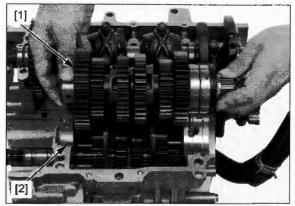
Remove the shift drum bearing setting washer-bolts [1].
