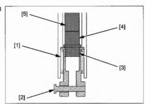
Apply molybdenum disulfide grease to the rotating area of a new needle bearing [1].
