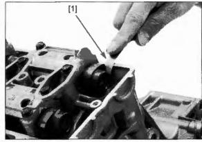
Turn the crankshaft clockwise 1/2 turn (180°), align the index line [1] on the CKP sensor rotor so that it is facing down as shown.
