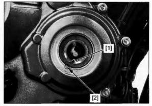
Make sure the timing marks ("IN" and "EX") on the sprockets are flush with the cylinder head surface and facing outward as shown.
